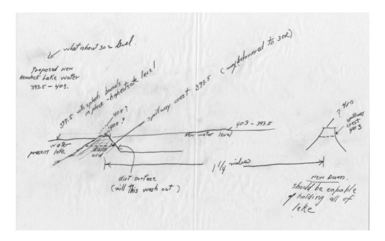
The spillway weir crest at the present Hemlock Lake dam is at elevation 393.5. The drop timbers in the spillway would be removed and the present Hemlock Lake dam retained, but with water at elevation between 393.5 and 403.00, water would stand at the same elevation above and below the dam, and the present spillway would no longer be used as a spillway but merely as an outlet channel.
